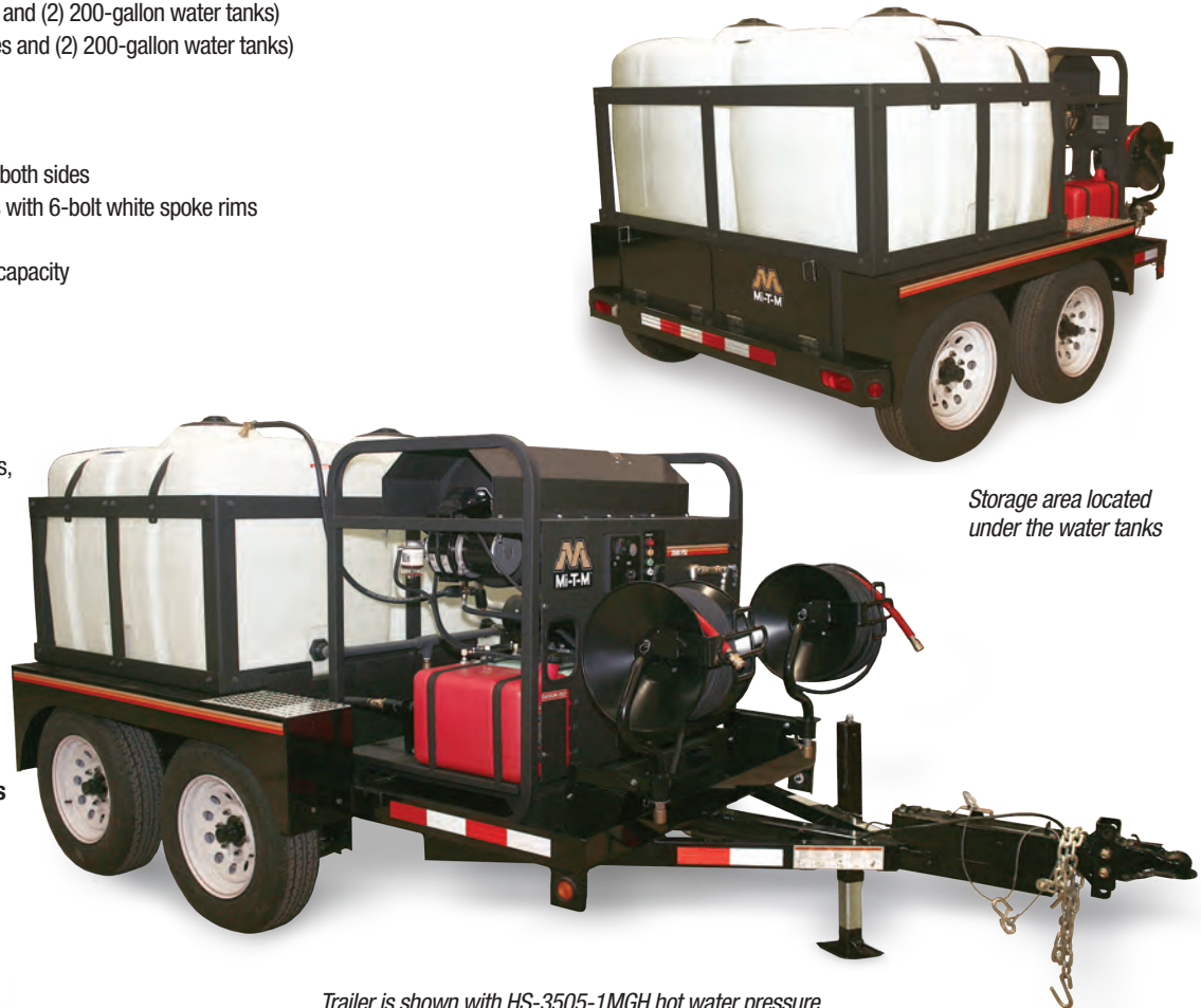
Trailer is shown with HS-3505-1MGH hot water pressure washer and hose reels (available as accessories)
