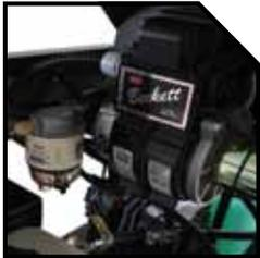
12 Volt Burner with fuel/water separator
